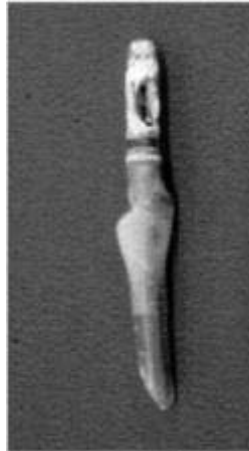
Fig. 1. A catheter that has undergone encrustation.
