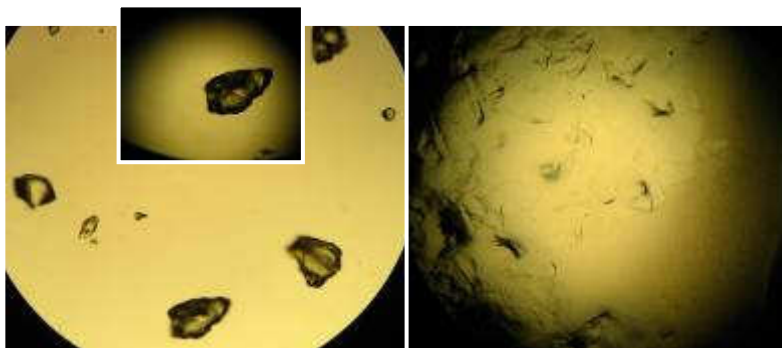
Fig. 9: On left: Solid 90-125 Bloom gelatin particles under 20X magnification (inset shows 40X magnified view). On right: Gelatin dissolved in acetate/citrate buffer under 20X magnification. Gelatin dissolved in 60°C water showed no irregularities, but rather, the solution appeared homogenous and translucent.
