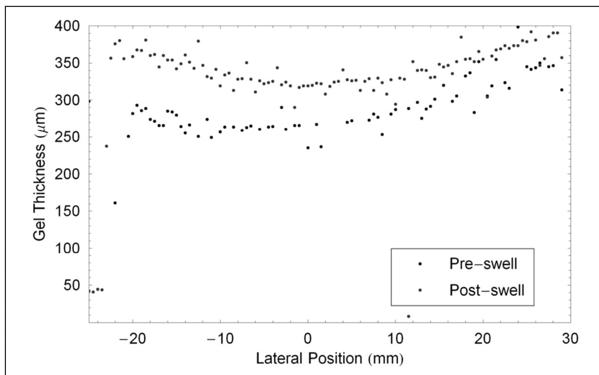
Figure 3: Thickness of pre-swelled (lower curve) and post-swelled (upper curve) hydrogel films as measured by ultrasound. Both curves are concave downward with the lowest value in the middle of the microscope slide.
