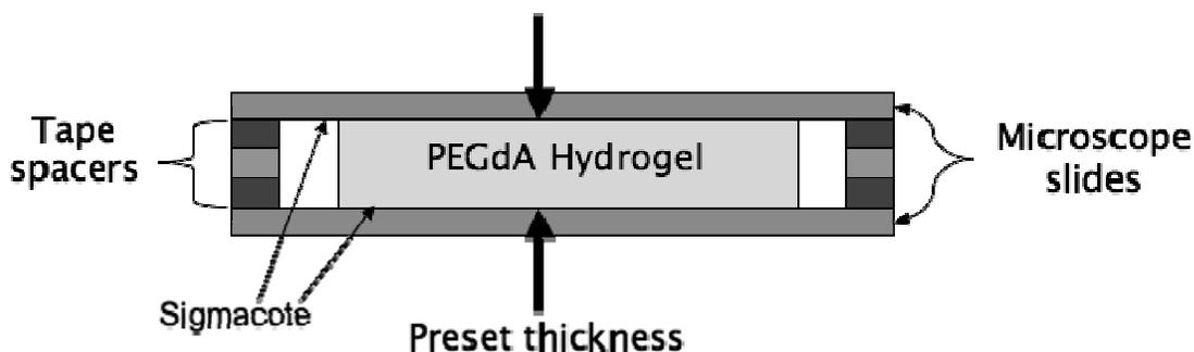
Schematic 1: Device to create thin PEGdA hydrogel films. The present thickness is determined by the layering of film and/or tape spacers.
