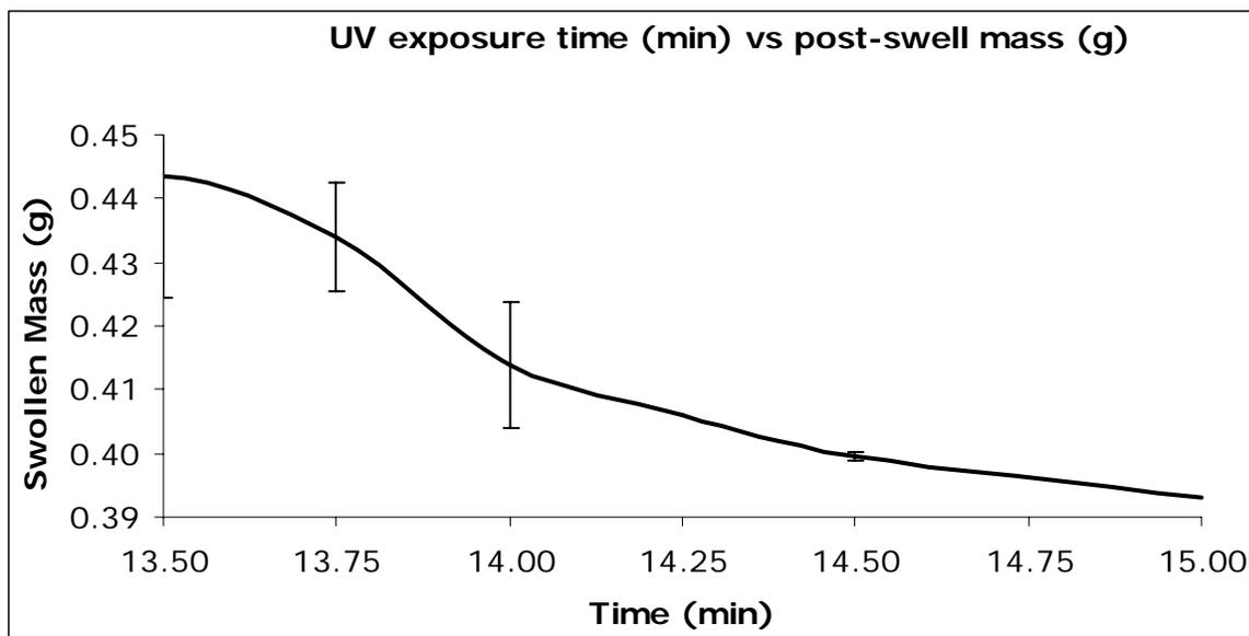
Figure 2: Effect of UV exposure time (13.5~15 min) on degree of hydrogel swelling. 14.5 minutes of UV exposure time was decided to be sufficient for photo crosslinking of PEGdA solution.
