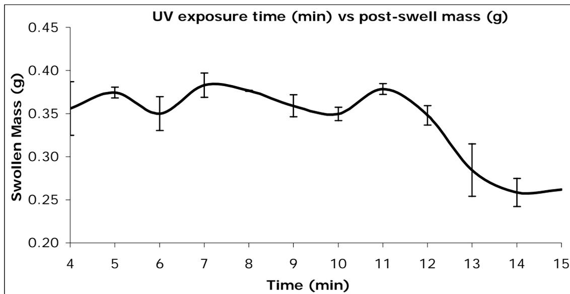
Figure 1: Effect of UV exposure time (4~15 min) on degree of hydrogel swelling. As UV exposure time increased, the degree of hydrogel swelling decreased. The swelling started to plateau after 13 minutes.
