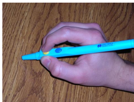
Figure 11: Squeeze stick. Clicks with the push of a button.
