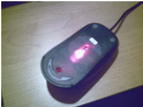
Figure 9: Reverse optical mouse design. Very sensitive, and easy to adjust.
