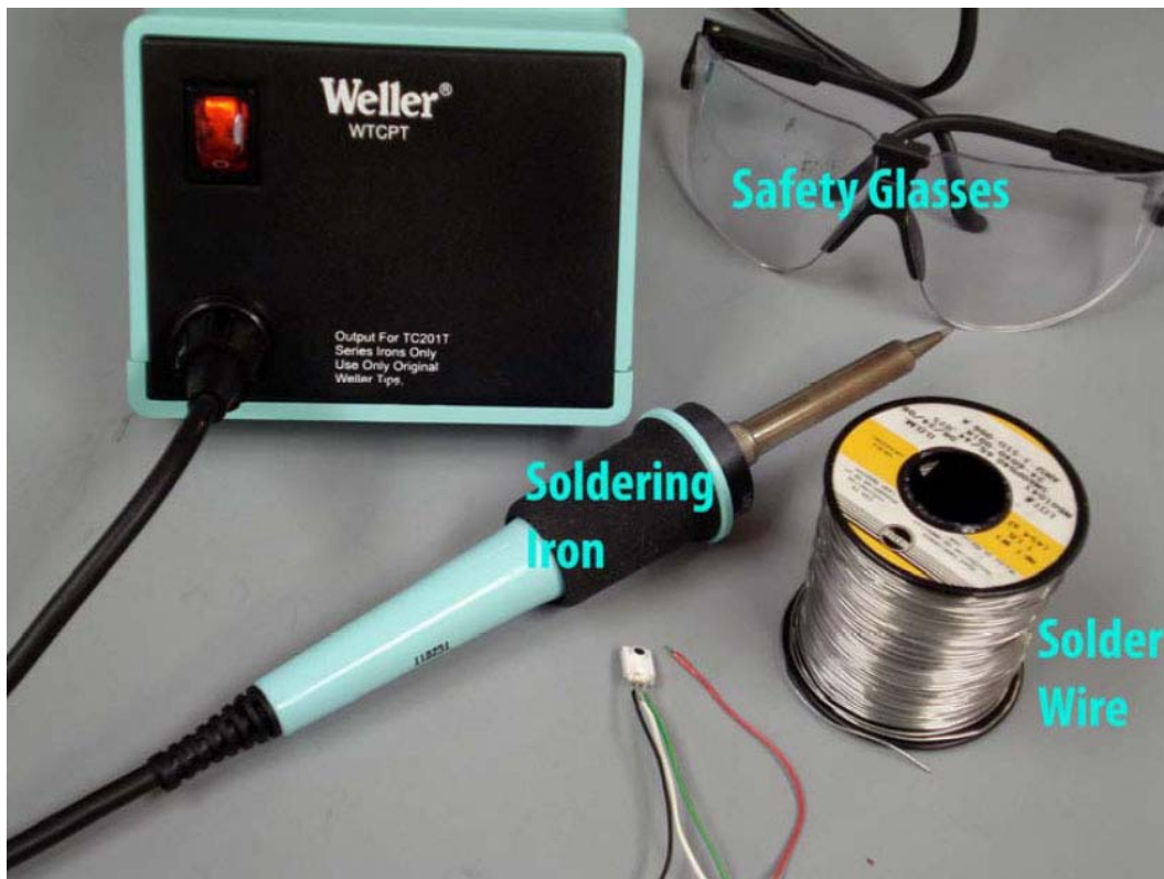
Figure 2 – Soldering equipment included in Tools You Will Need to build the sensor.
