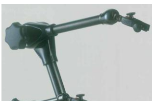
Figure 6 - Several Articulated Arm models. One knob at the corner joint tightens all three joints, allowing size degrees of freedom with one adjustment. From Noga Engineering.
