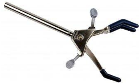
Figure 8. A 3 pronged clamp that could be used to hold the probes in position. The two screws are used to tighten the clamp when it is in the correct position.
