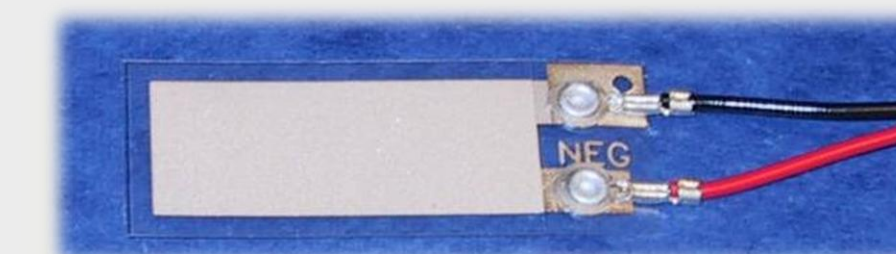
Fig. 4 Piezoelectric film with rivets [4]
