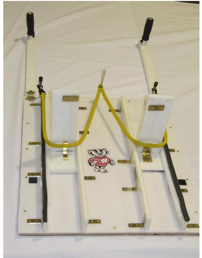
**Figure 4:** MRI-Compatible Exercise Device. Above: Subject is placed in the device. Handles provide both torso stability and device stability. Right: Device shown alone.
