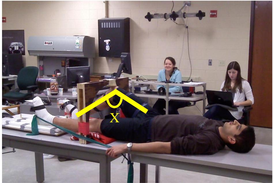
**Figure 2:** Motion Capture Setup. Motion capture markers were placed at the foot, shank, and thigh to track movement of the lower extremity. Tibial femoral joint angle was measured.
