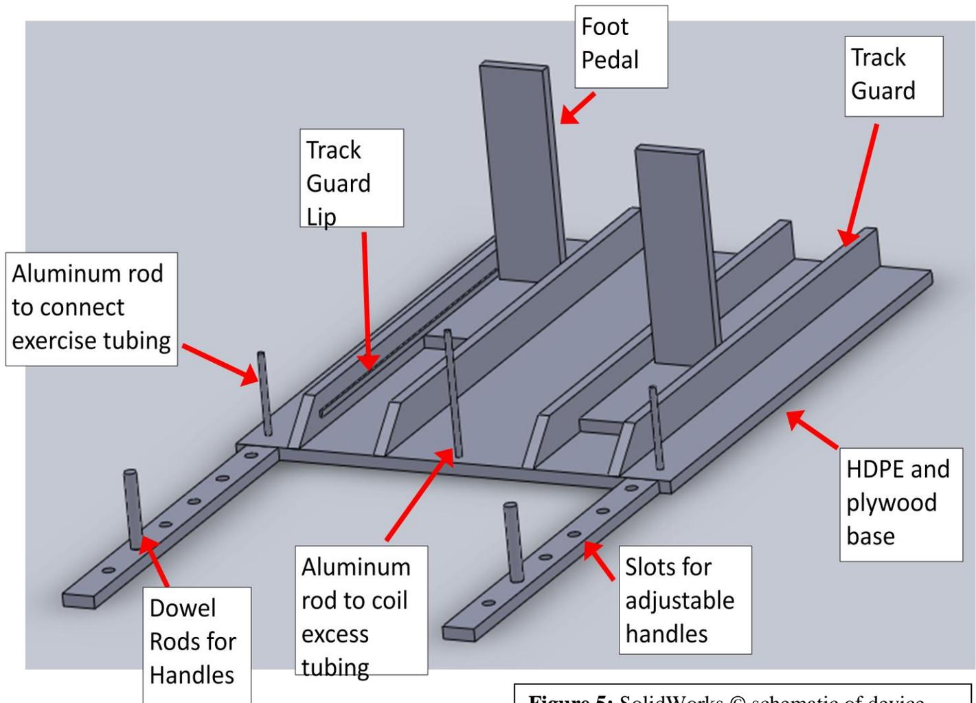
**Figure 5:** SolidWorks © schematic of device.
