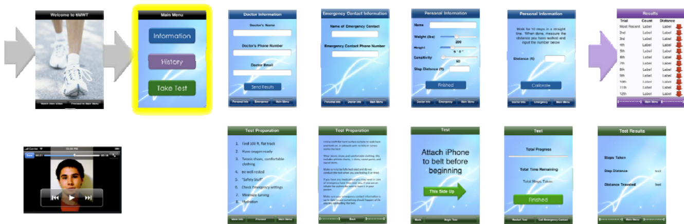
Figure 4: Above is final flow design chosen based on results of usability testing. Program is entered from the left-top corner and the yellow highlighted page is the main menu. The blue, green, and purple arrows represent offshoots from the main menu and represent the information storage, testing, and history pages of the application respectively.
