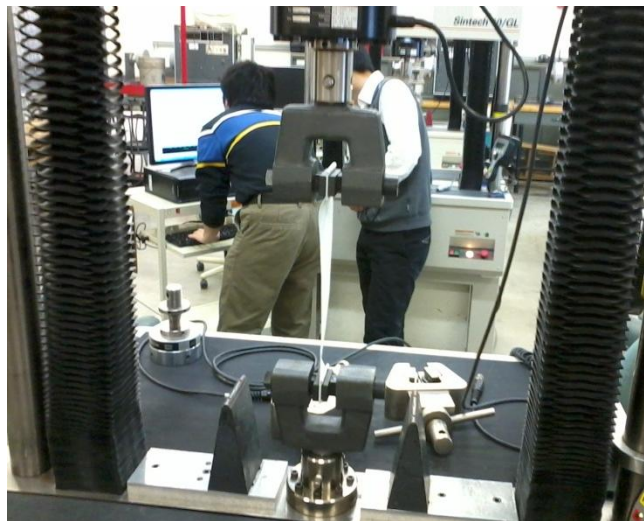
Figure16: Tensile test performed using a MTS Sintech Universal Testing Machine on the elastic wrap material.
