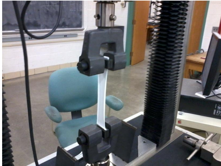
Figure 15: Tensile test performed using a MTS Sintech Universal Testing Machine on the spandex material.
