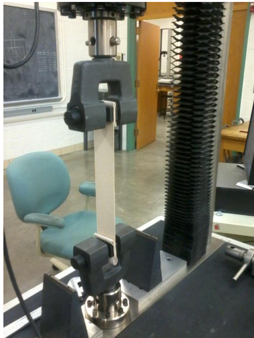
Figure 14: Tensile test performed using a MTS Sintech Universal Testing Machine on the ACE bandage.
