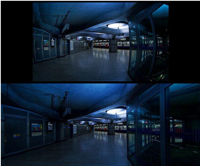
Figure 3: Top-image taken using a fisheye lens; Bottom-Image taken using a non-distorting lens Source: http://en.wikipedia.org/wiki/File:Panotools5618.jpg
