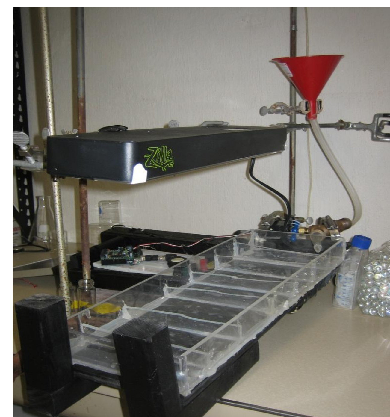
Figure 9: Experimental set up with uv source running parallel with Plexiglas box at a 6° angle
