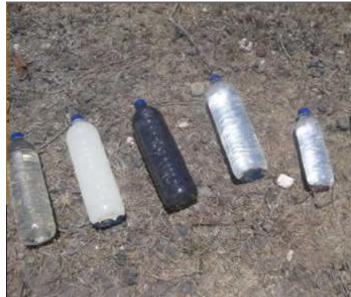
Example of water bottles coated with \text{TiO}_2
