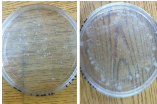
Figure 8: TiO 2 + uv (left) and uv (right) effect on bacterial regrowth using BrightWater prototype.
