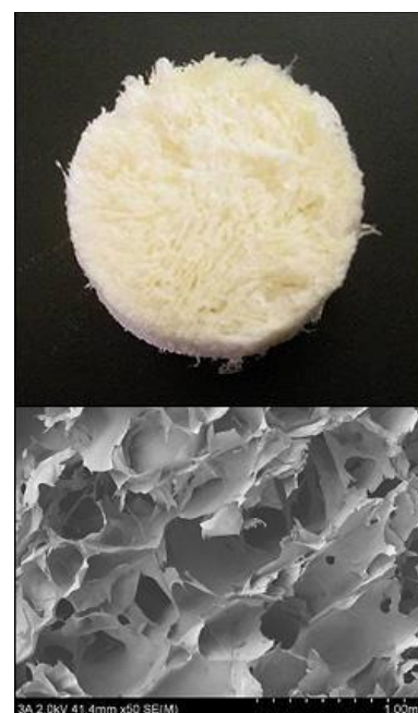
Figure 7: Dry alginate scaffold (top). Microstructure of dry alginate scaffold (bottom) [26].
