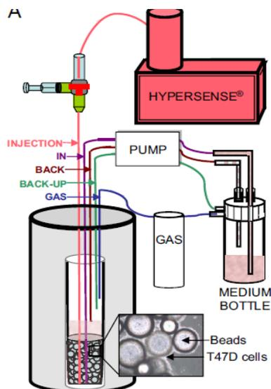
**Figure 2: Diagram of bioreactor system including injection and output lines for cell media and gases. A scaffold that consists of many microscopic beads is contained within this bioreactor [3].**
