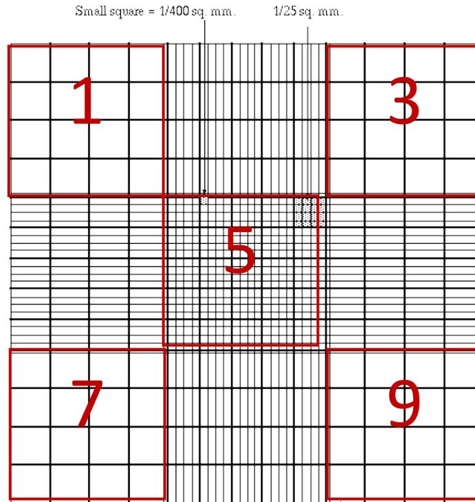
Figure 1: Grid of hemocytometer showing the numbered squares which should be counted.
