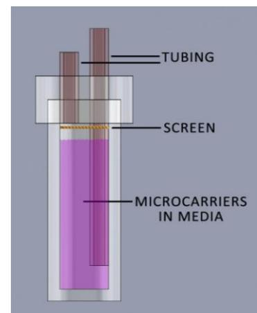
Figure 12: Design of bioreactor cartridge using SolidWorks by bioreactor team, edited to include filter and media. 17
