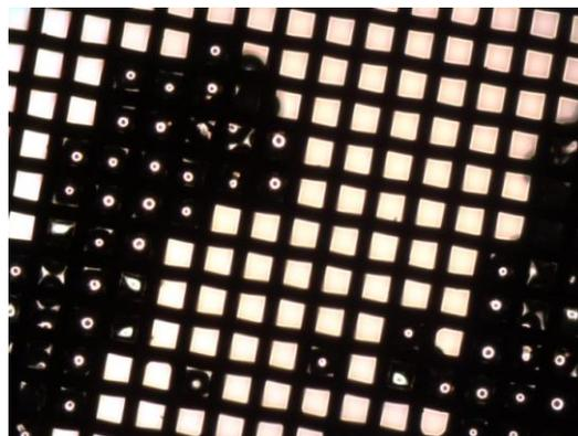
Figure 13: 106 micron mesh size, brass filter under 10x magnification.
