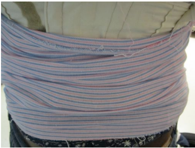
Figure 4. Original belly band after movement tests displays a high degree of rolling and bunching
