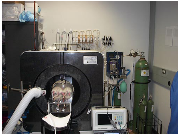
Figure 1: This picture shows four rats in the PET scanner at the client's laboratory. The rats are oriented in a two by two square [Ho, J. et al.].
