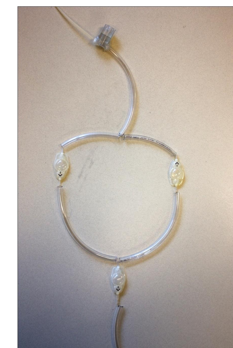
Figure 7: The Medtronic valves are pictured in the testing loop above.
