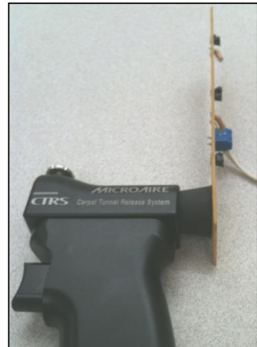
Figure 9. The circuit board is attached to the back of the endoscope shell by a rubber cap. The Wii remote views the LEDs from behind the endoscope working view.
