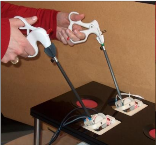
Figure 4. (left) displays the TrEndo surgical simulation system. The handheld endoscopic instruments mechanically couple with a device that uses optics to detect movement ( www.ncbi.nlm.nih.gov/pmc/articles/PMC2211365/figure ). Figure 5. (right) displays the set-up for TrEndo simulation system. The instruments allow for advanced haptic feedback throughout the surgery ( www.ncbi.nlm.nih.gov/pmc/articles/PMC2211365/figure ).
