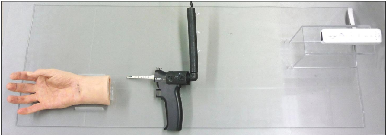
Figure 15. Final prototype with the acrylic platform housing (from left to right) the hand model, the endoscope with blade attachment, the LED circuit, and the receiver.
