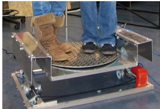
Figure 8 – Picture of final design, shown with ~270lb loading
