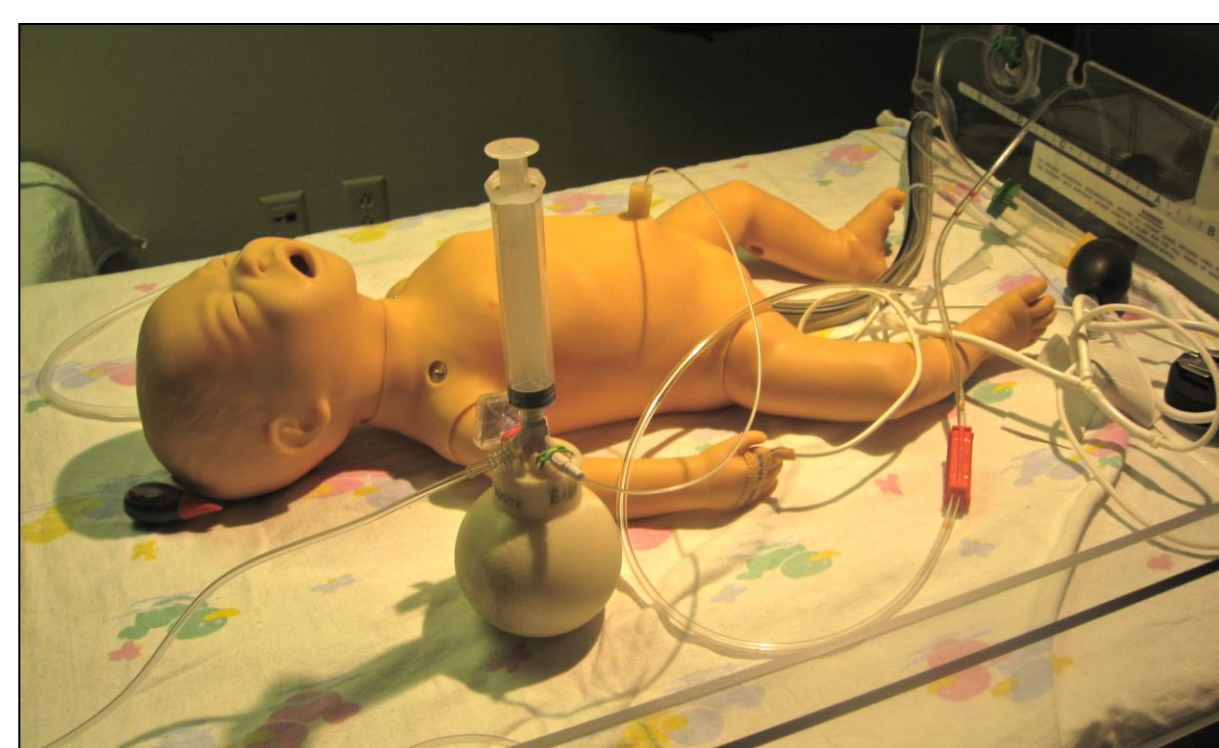
Figure 3: The stopcock base next to the baby on a typical patient bed. The baby is completely covered during the procedure and space limitations are an important consideration to the design.
