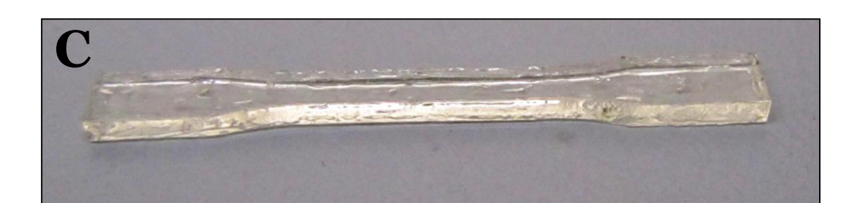
(B) MTS Criterion Model 43 used for tensile testing (C) Tensile test specimen with dimensions specified by ASTM D638-10
