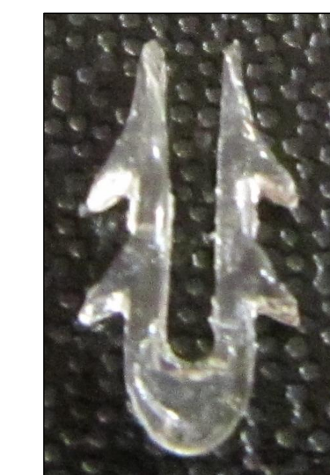
Figure 7: Staple after being cut with laser cutter
