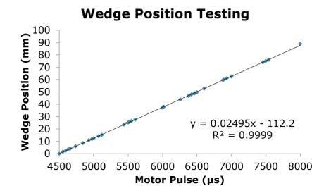
Figure 7: Wedge Positioning
