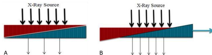
Figure 1: Wedge-Based Beam Attenuation
