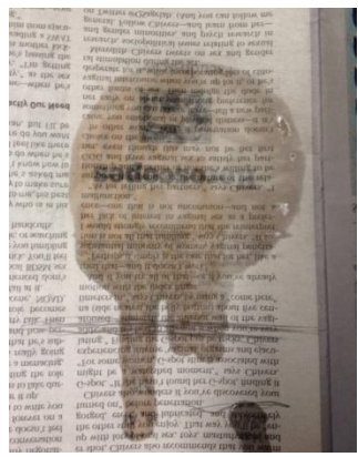
Figure 17. Spray pattern on the newspaper for the first test.
