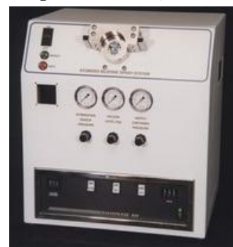
Figure 5. Automatic silicone oil spray chamber (McClellan Automation Systems, 2011).
