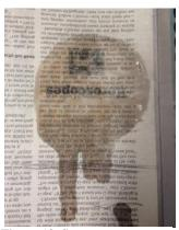
Figure 18. Spray pattern on the newspaper for the first test.
