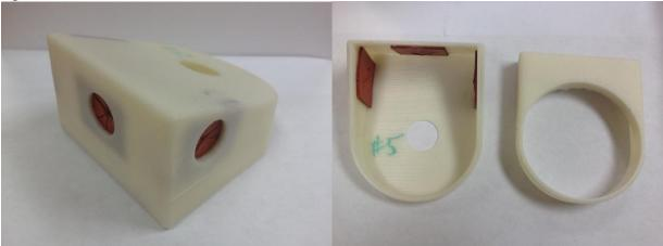
Figure 17. Demonstration of the fifth prototype. The left picture shows that the two pieces snaps together, which gaskets attached to all 3 holes. The right picture shows that the two pieces can be separated.
