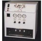
Figure 5. Automatic silicone oil spray chamber (McClellan Automation Systems, 2011).
