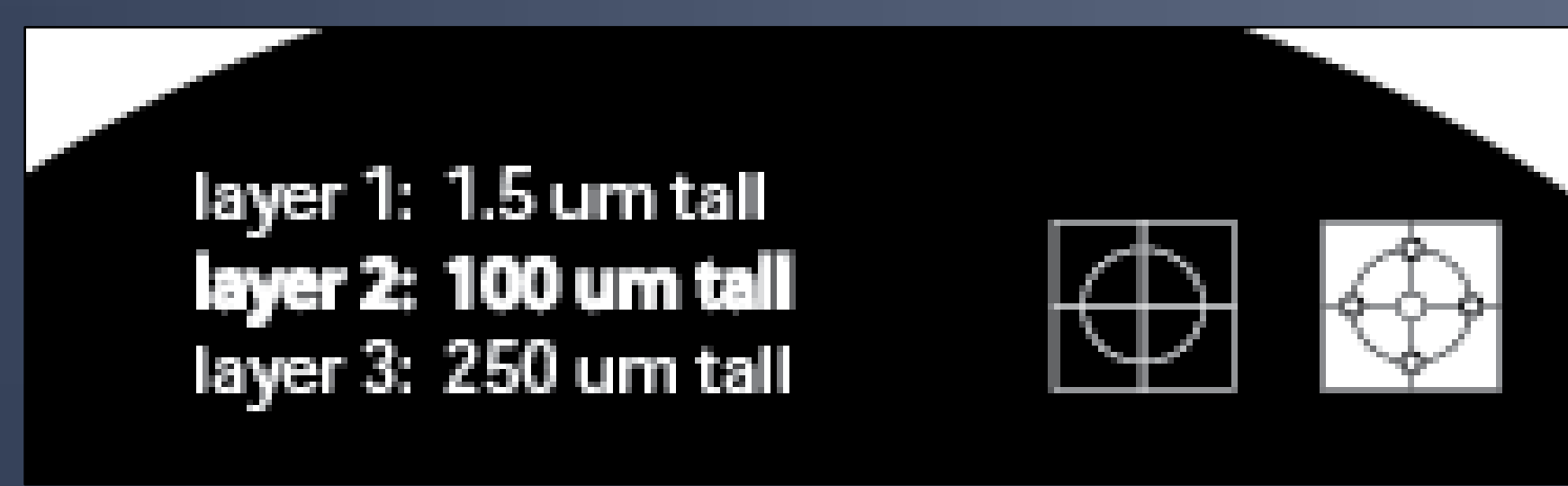
Figure 1: Photomask alignment marks used for manual alignment by eye [4].
