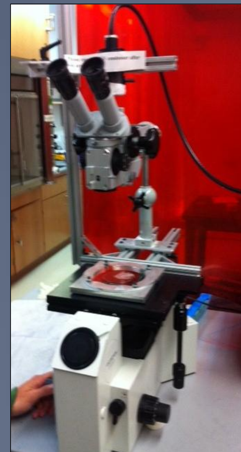
Figure 2: Microscope assisted aligner as seen in Professor Williams' photolithography lab.
