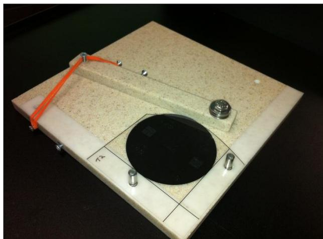
**Fig.1: The final prototype of the low-cost aligner in use with wafer constrained and photomask placed over alignment pins.**
