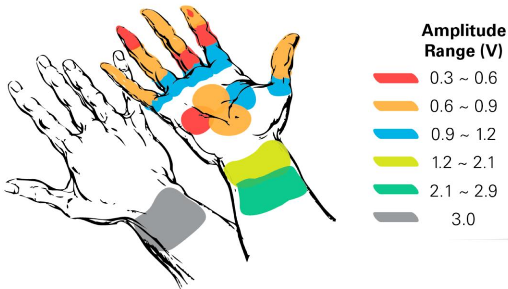
Figure 14: Map of hand sensitivities based on applied factor voltage: Notice that there is an increased sensitivity at the tips of the fingers [Adapted from 7].
