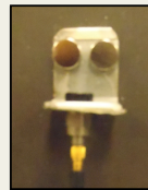
Figure 6 (above). Method of attachment. Aluminum angle bracket is used to position accelerometer in the correct orientation. Neodymium magnets are used to secure to treadmill.
