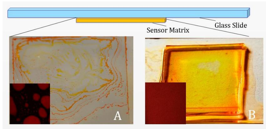
**Figure 9: Image A is the Rudpp sensor incorporated (via soaking) onto a polystyrene matrix and Image B is the Rudpp sensor incorporated onto a PDMS matrix.**
