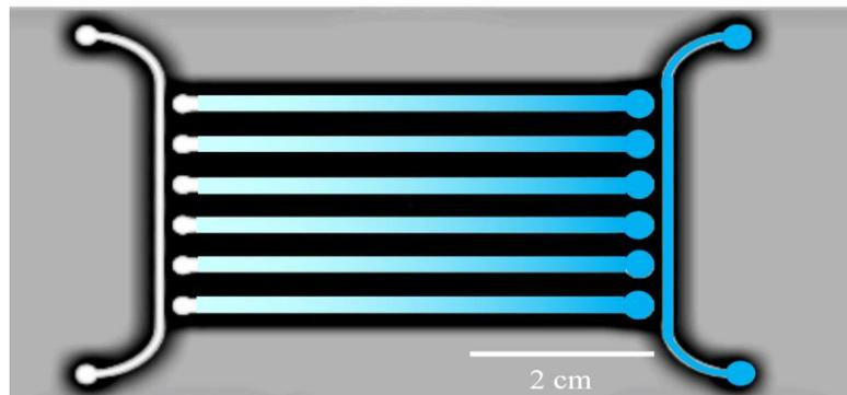
**Figure 4: The design of the microfluidic device. Oxygen (blue) flows through the right-hand channel and diffuses to the left, creating a decreasing gradient. Nitrogen (white) flows through the left-hand channel.**
