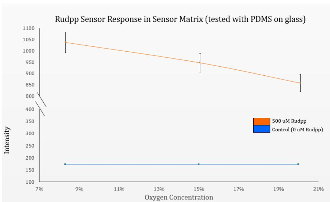
**Figure 12: Sensor molecule response curve, best fit curve**
