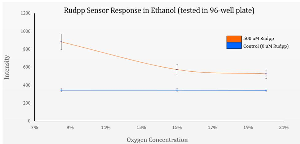
**Figure 11: Sensor molecule response curve, best fit curve**
