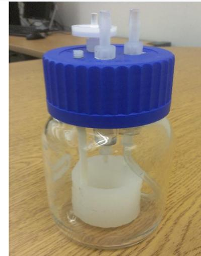
Figure 3. Final assembled bioreactor with modified cap for inlet/outlet ports, air filter, and polypropylene ovary holder funnel.
