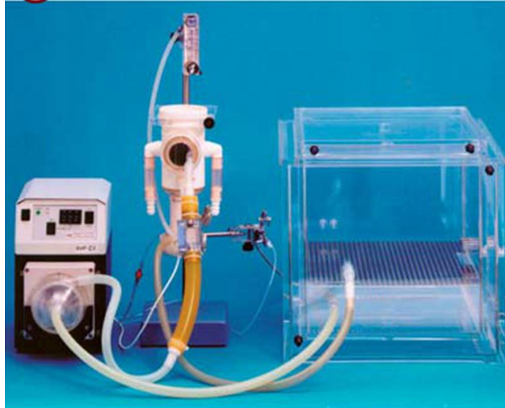
Figure 3. Example of bioreactor used for a pig kidney [10].
