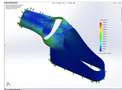
Figure 3: Von Mises stress for the shoulder strap.
