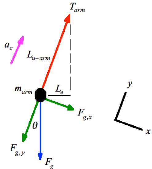
Figure 4: The free body diagram depicting the mass of the pendulum and corresponding forces at any given angle from the vertical to the mass.
