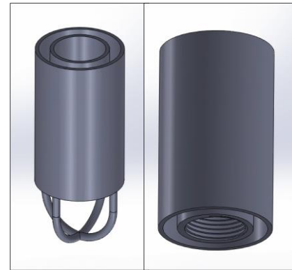
Figure 5: SolidWorks renderings of a) free sliding bottom cap with hooks for fixation; b) threaded top cap that supplies compressive load when centerpiece is twisted by moving down the centerpiece toward the end cap.
