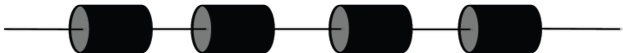
Figure 7: Schematic representation of threaded segments design. The threaded segments from the carjack design are strung along a stainless steel wire.
