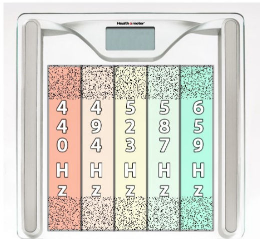
Figure 6: Conceptual diagram of second proposed design. Left/right feedback would be constant, but the plate would vibrate in the front and the back when weight distribution shifted too far in the respective directions. The tones and plate vibrations could occur simultaneously for a more consistent feedback. The subject should not feel any vibration when within the threshold for front/back balance.
