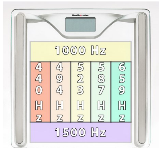
Figure 5: Conceptual diagram of first proposed design. New zones were added to the front and back of the scale to indicate a new tone that overrode the five left/right ones. The left/right tones would not play when the subject’s weight distribution goes beyond the threshold for front/back balance.
