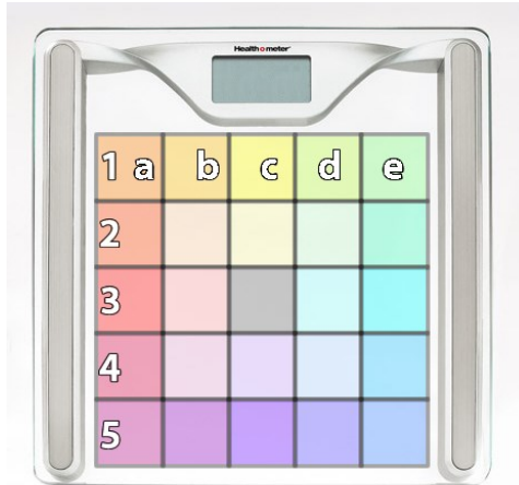
Figure 8: Conceptual diagram of fourth proposed design. The scale would divide vertically just as much as it would horizontally, resulting in a grid of 25 zones. Each zone would be assigned two tones depending on left/right (a-e) and front/back (1-5) positions. When the subject's center of gravity was in a particular zone, both of its tones would play simultaneously, resulting in a unique sound for each zone. This functionality would be similar to a touch-tone telephone.
