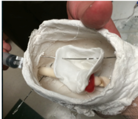
Figure 1: Dr. Halanski's initial prototype. The model is made from a plaster mold. The inside of the model is hollow so that a balloon containing fluid can be placed [3].
