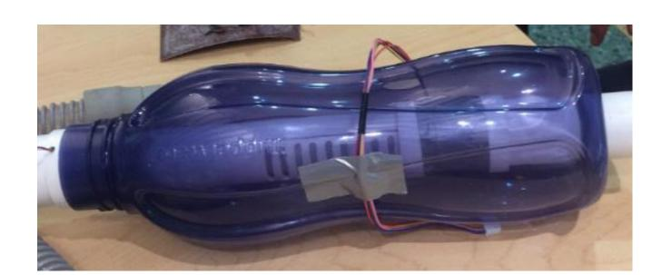
Figure 2. A hard waterbottle with PVC pipe through it was used as the body of the device. The PVC pipe has slits cut into it to vary dead space volume
