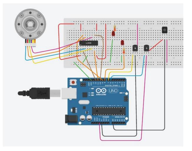
Figure 5. A schematic of the circuit that controls the stepper motor based on the readings from the flow sensor.
