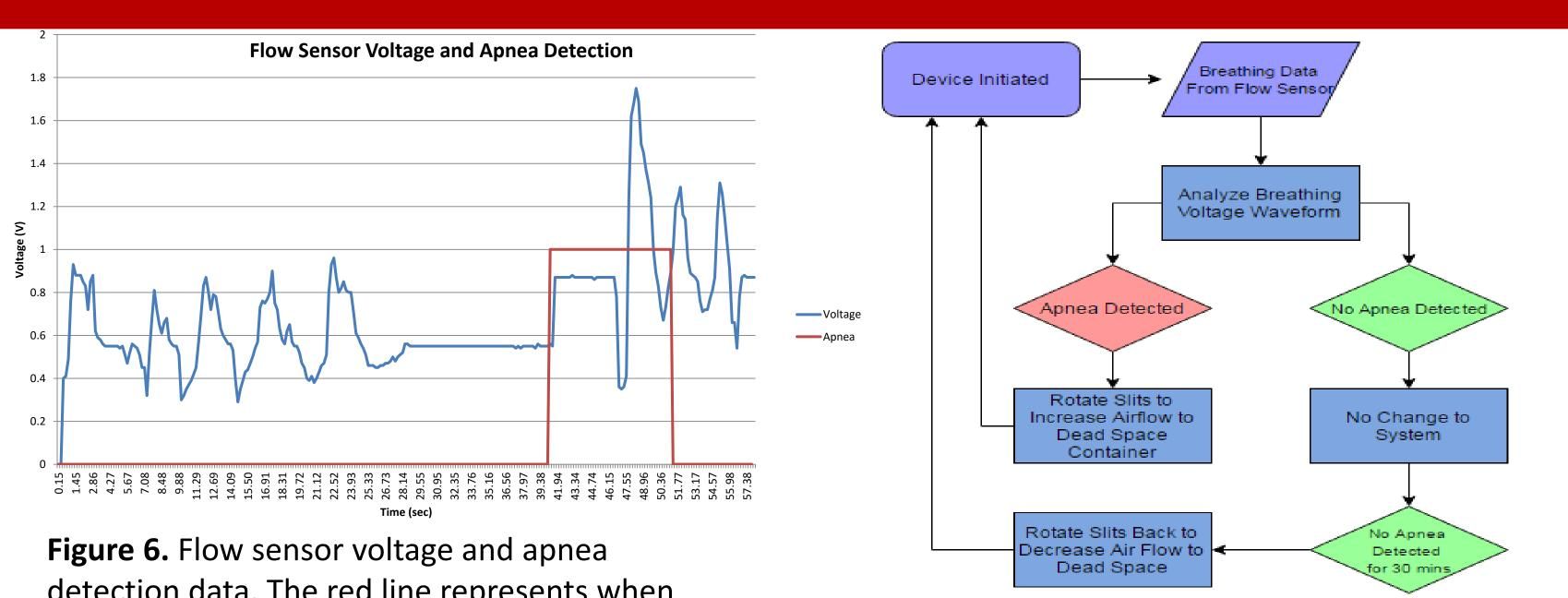
detection data. The red line represents when apnea was detected and the blue line represents the breathing pattern of the test subject. Testing verified the functionality of the algorithm.
