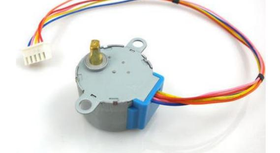
Figure 4. A stepper motor is secured at the end of the PVC pipe. It is connected to a cover slide that rotates to cover or uncover slits cut in the PVC pipe.
