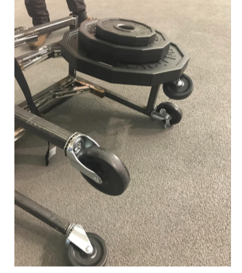
Figure 11. Chair Leg Strength Functional Load
