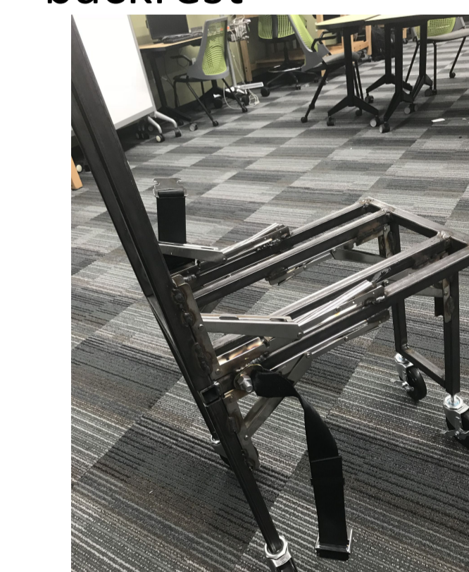
Figure 5. Locking hinges attaching the seat to the backrest
