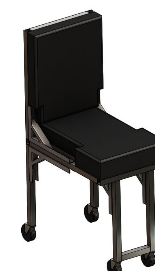
Figure 6. Steel frame of chair
