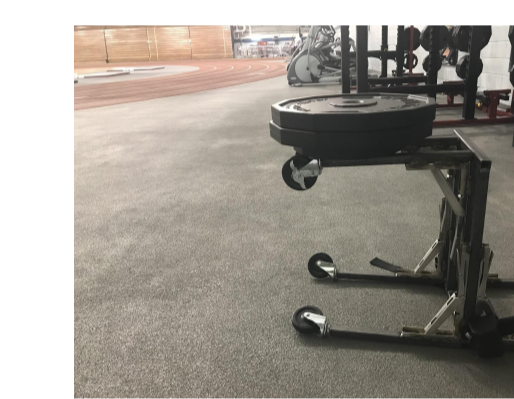
Figure 9. Chair Leg Strength Proof Load
