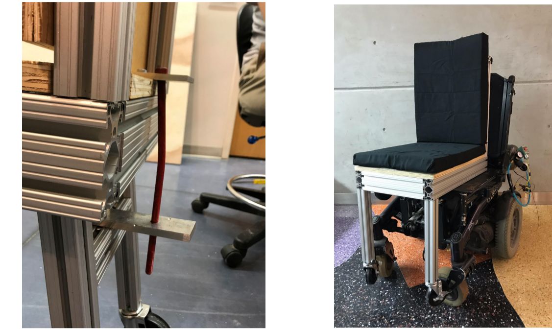
Figure 2 & 3. Fall 2017 prototype close up of locking mechanism and final prototype on an electric wheelchair
