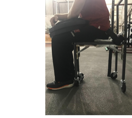
Figure 10. Chair Drop Proof Load Test
