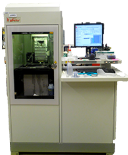
Figure 8. Viper SLA 3D printer at Morgridge Fabrication Lab. Layers of resin are photocured into the 3D design, with a high precision laser.
