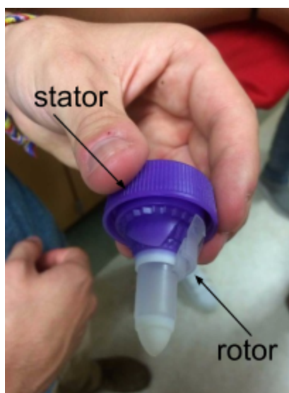
Figure 2. Conical Tube used with grinding teeth used in the gentleMACS™ system to dissociate tissue.
