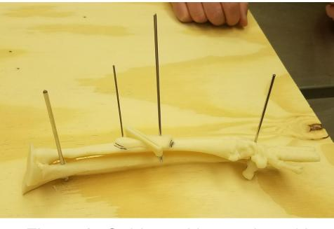
Figure 9: Guide and bone pinned in place for cutting
