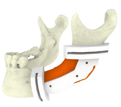
Figure 11: Cutting guide model made by Xilloc for practicing mandibular surgery<sup>[4]</sup>
