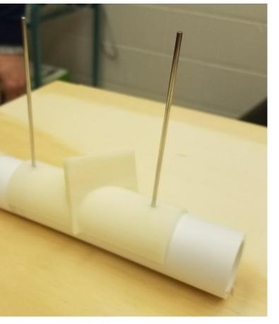
Figure 7: Guide pinned to testing jig
