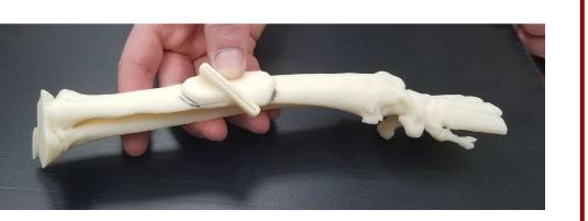
Figure 8: 3D printed bone and guide
