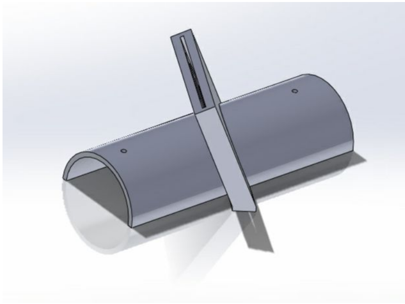
Figure 7: 3D model of the current test specimen which includes compound angles to simulate actual surgical cuts.
