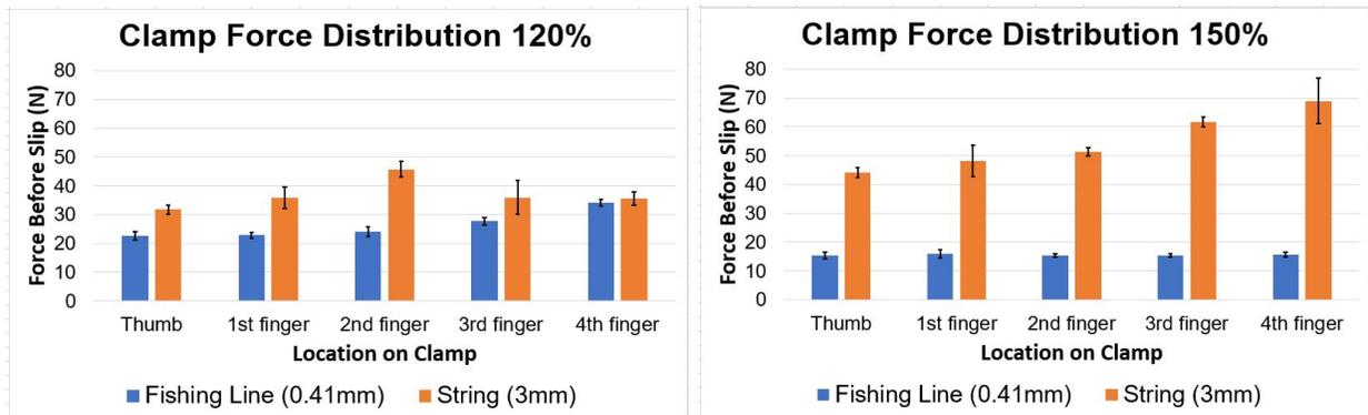
**Figure 4:** Results of clamp failure testing for a) the 120% size hand and b) the 150% size hand.
