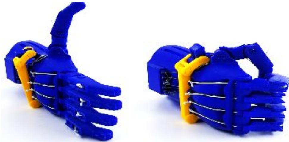
**Figure 1:** Photos of the Raptor Locked and Reloaded with the clamp open (left) and the clamp engaged (right).
