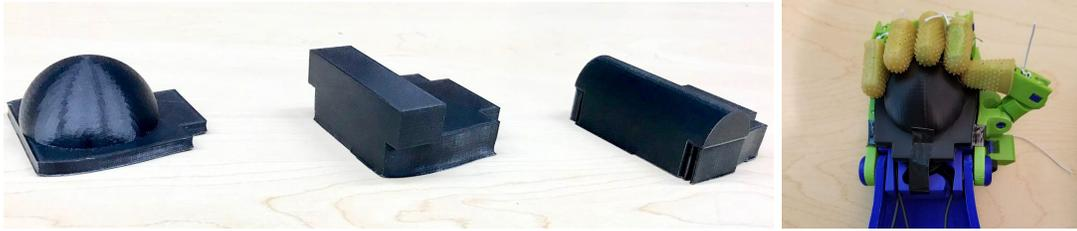
**Figure 2:** Left to right hemisphere, block, and cylinder used for the maintained object force testing. Image on far right shows an example of the data acquisition set up for the hemisphere.
