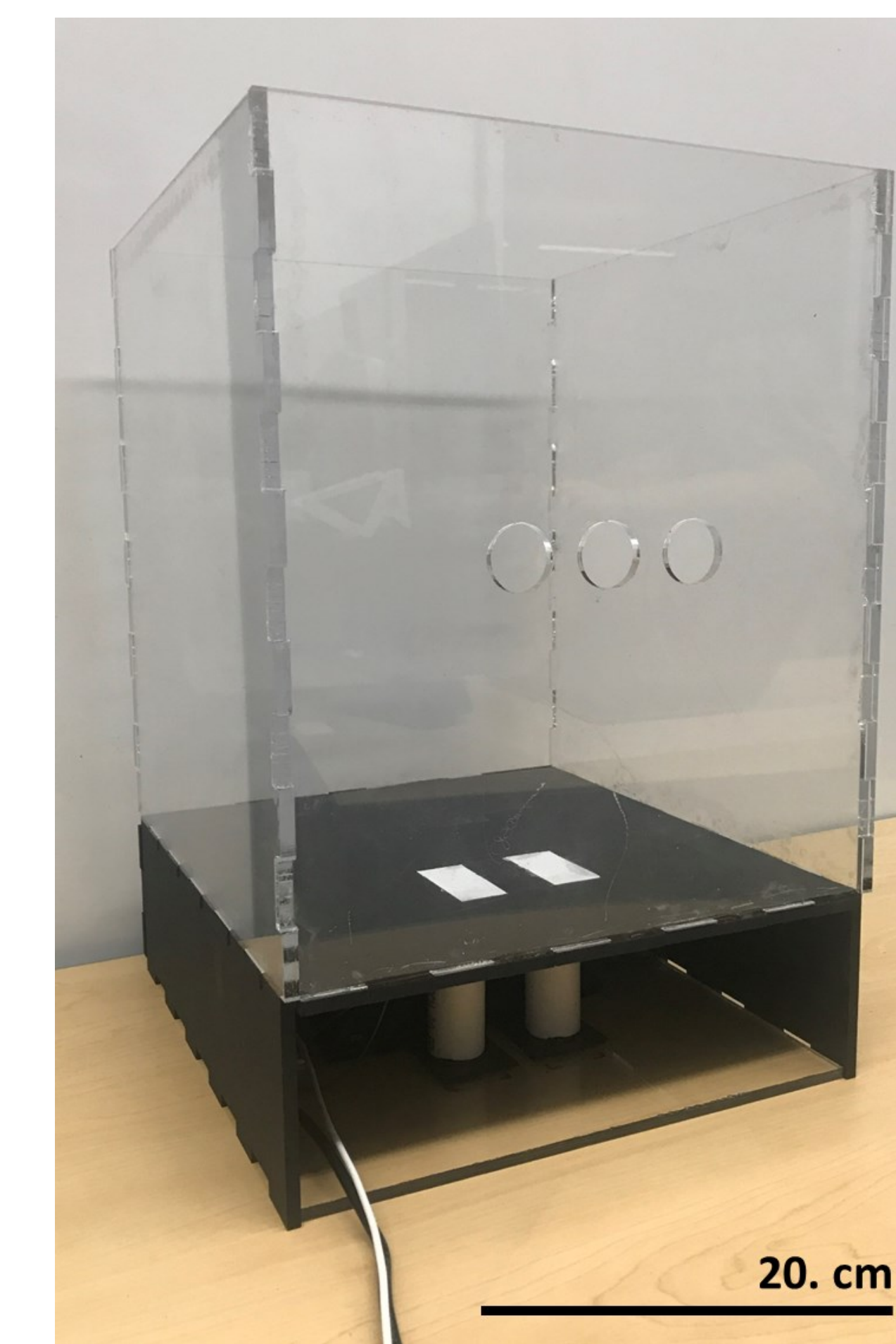
Figure 7 (Left). A plexiglass cage with holes cut out of the bottom where the transducers will couple with rubber mat on the bottom of the cage. Included in the cage is a water resistant rubber mat in case of rodent waste. Additionally, the circuitry and transducers will be safe from harm underneath the cage, with the only cords coming out of this section of the enclosure being an 3.5 mm headphone jack, as well as a power cord for the amplifier. The transducers are also in this bottom section of the enclosure where they are coupled to the rubber mat due to the cement and PVC standoffs built for them so that the transducers fit properly into the platform cutouts in the bottom of the cage.
