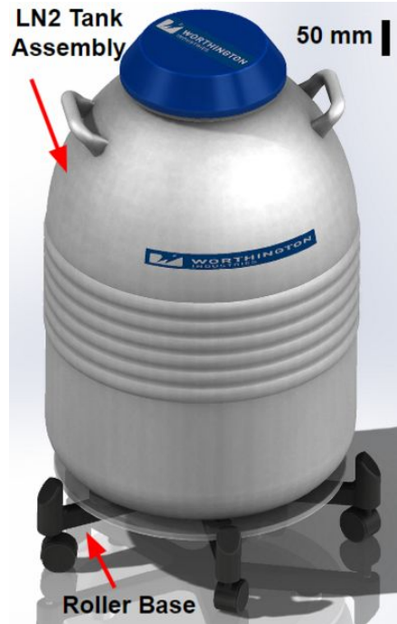
APP Figure 1: SolidWorks rendering of the fully assembled roller base and integrated scale with the LN2 tank placed directly on the assembly.
