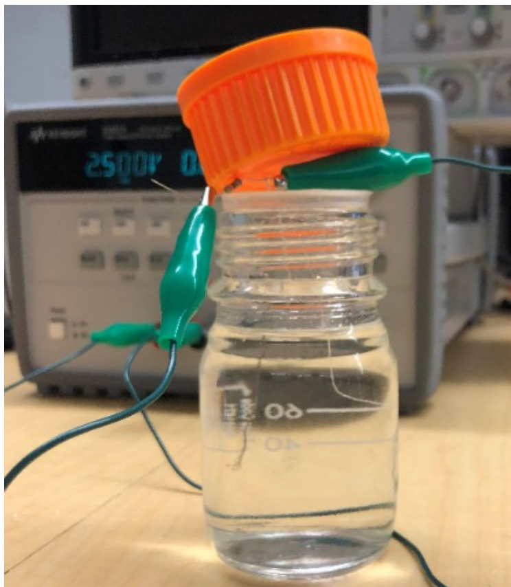
Figure 2: The setup of the electrodeposition of Ag/AgCl electrode
