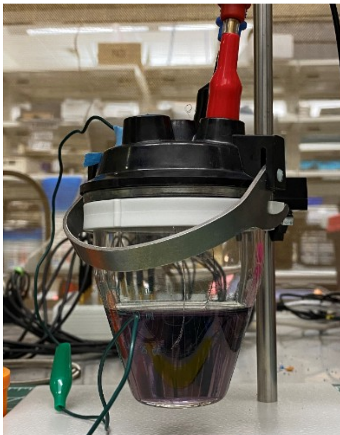
Figure 1: The set up of the electrodeposition of IrOx.
