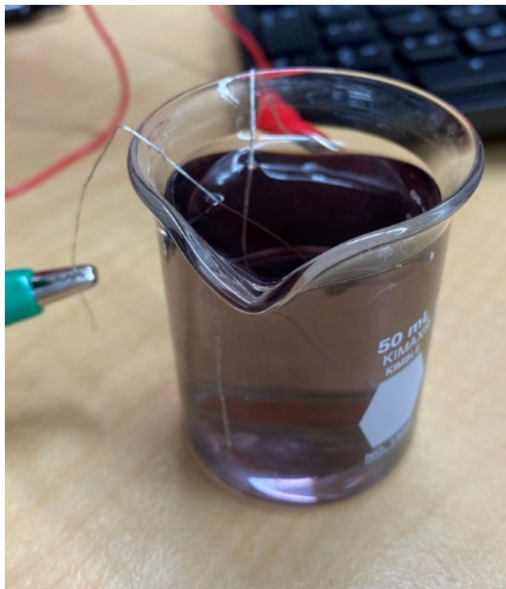
Figure 1: Two wires of Pt/Ir were immersed in the electrodepositing solution and connected to the power supply by alligator clips.
