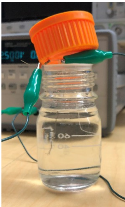
Figure 2: The setup of the Ag/AgCl electrodeposition
