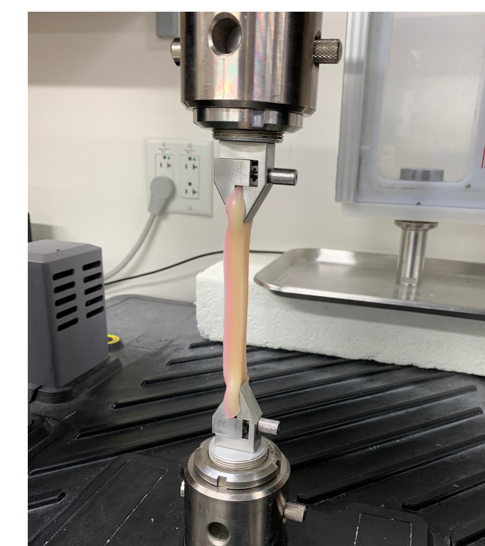
Figure 7: Silicone strip being tested in tension in the MTS machine.
