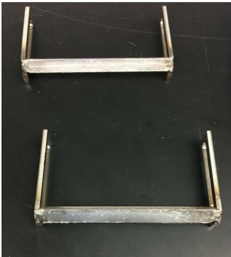
Figure 4. Bottom faces of the device immediately after a thin layer of silicone was applied.
