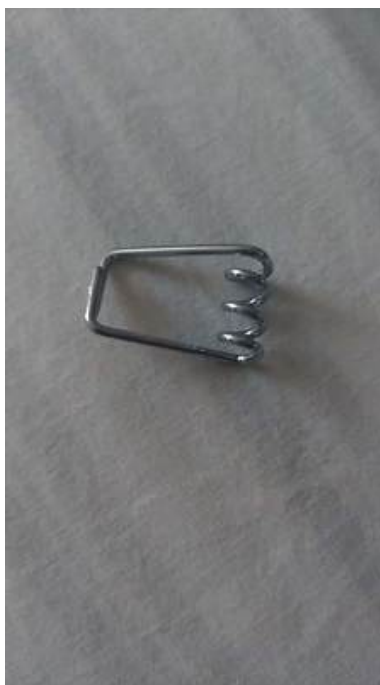
Snapchat-1759040113.jpg(139.9 KB) - download Images of the torsion spring when assembled and unassembled from the clothespin.
