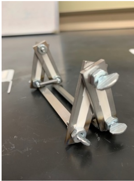
Figure_2.jpg(69.4 KB) - download Figure 2. The slot fillers were press-fit into the slots, securing the thumb screws in place at the ends of the slots.
