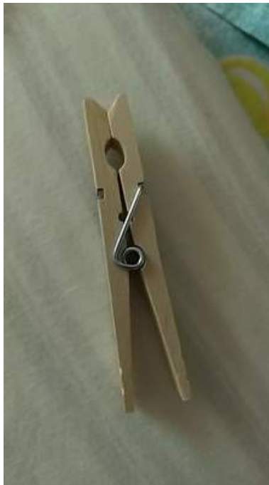
Snapchat-1996034171.jpg(40.8 KB) - download Images of the torsion spring when assembled and unassembled from the clothespin.
