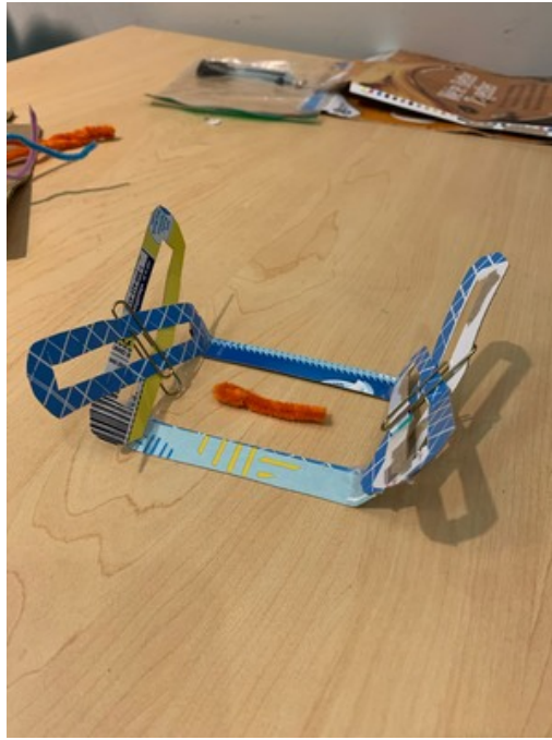
_private_var_mobile_Containers_Data_Application_8527CA1F-1A83-458F-8720-6111AB980B7E_tmp_E321E19B-AA8B-4555-B0AA-40FB095 DE6C4_Image.jpeg(1.7 MB) - download Figure 1: Cardboard prototype of the current design. The orange pipe cleaner is the wound location relative to the device. The cardboard prototype was constructed with incorrect dimensions and is not to scale of the final design. The two raised sides of the device are adjustable and can bring the long sides against the skin closer together during approximation. The adjustable sides can then be fastened into position with a wing nut or other fastener (the paperclips in the prototype simulate the fasteners).
