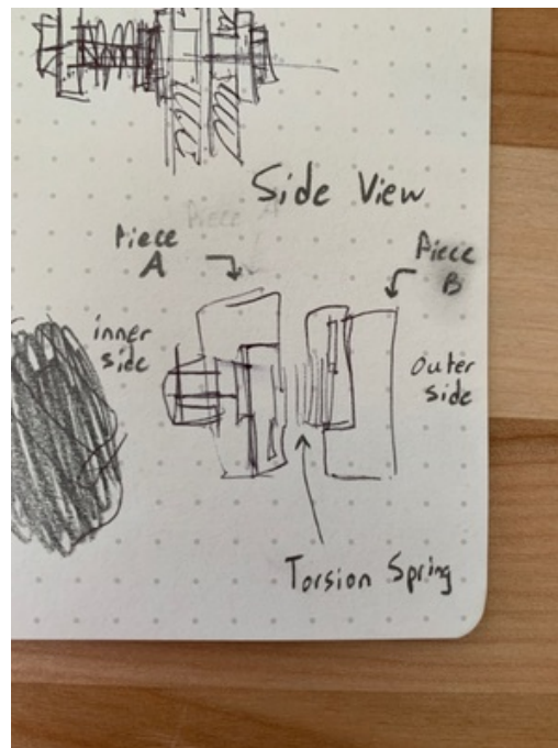
3E516548-B736-4B33-B9ED-F1373B946055.jpg(131.7 KB) - download Pieces A and B secure torsion spring
