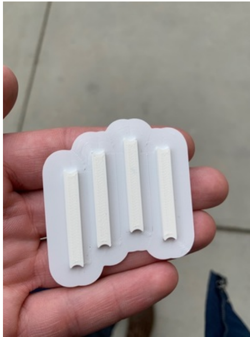
Figure_1.jpg(80.4 KB) - download Figure 1. Option 1 slot fillers right after 3D-printing.
