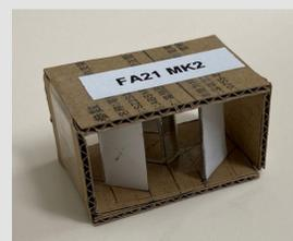
Figure 2: Early proof-of-concept prototype design utilizing a double-mirror array fabricated from cardboard.
